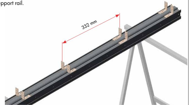
6. Attach UPM ProFi Quiet Tape into the designated top grooves of the support rails.
