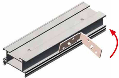
1. Build a subconstruction framework with **Corner Piece**
